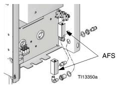
Fig. 60: Air Flow Switches
